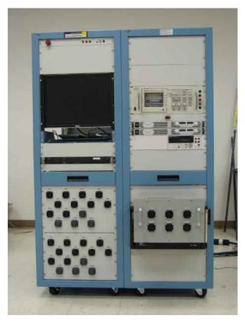
The Cargo Handling test station is designed for the evaluation of control units used to configure and place pallets on a cargo plane. The test station creates a simulated work environment to verify if the control units are functioning correctly. Failures can be quickly identified and prepared for repair.
