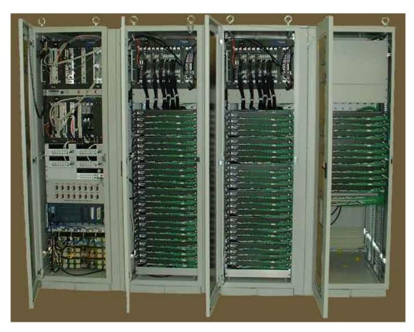
DAQFE is a high speed data acquisition system that utilizes fiber optic and copper LAN technology for data transfers. The system is designed to have a large number of channels with minimal latency and no data loss.
