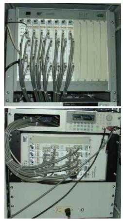
The LMDAS is a single bay VXI based data acquisition system designed to provide measurement capabilities for 48 thermocouples, 64 voltage measurements, 56 strain gage channels and a tachometer channel. Sensor measurements are acquired and stored in real time. The strain gage and voltage channels can be sampled at rates up to 40KHz. LMDAS allows essential data output required by the user to be quickly compiled, edited and exported.
